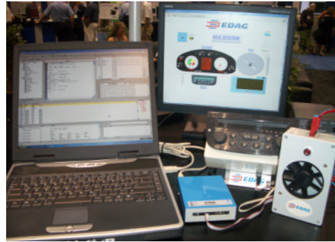
LabVIEW and winIDEA running together on a two-screen PC system, interfaced to EDAG's embedded target with the iSYSTEM iC3000 On-Chip Debugger.
